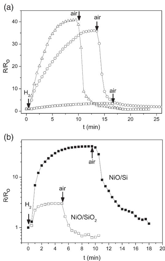
Fig. 2. Dynamic response characteristics of NiO thin films exposed in 3%  $H_2$  in air mixture: (a) films deposited on (001) Si at working temperatures of 150 °C ( $\square$ ), 180 °C ( $\circ$ ) and 210 °C ( $\triangle$ ); (b) comparison of dynamic response characteristics for films deposited on (001) Si and  $SiO_2$  substrates at 210 °C.  $H_2$  mixture application started at 0 min and ceased at each curve's maximum.
