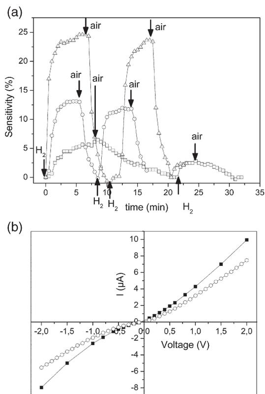
Fig. 3. (a) Dynamic response characteristics of Au/NiO/Si Schottky diode exposed in 3% H<sub>2</sub> in air mixture at working temperatures of 70 °C (Δ), 50 °C (○) and RT (29 °C) (□) and at forward bias of 2.4 V. (b) I–V characteristic at 29 °C of the Schottky diode in air flow (■) and in the presence of 3% H<sub>2</sub> in air mixture flow (○).
