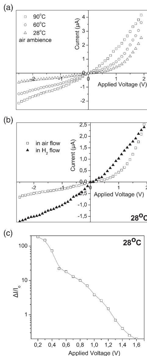
Fig. 4. (a) I–V characteristics of n-SnO<sub>2</sub>/p-NiO on (001) Si hetero-structure at 28 °C, 60 °C, 90 °C, in air ambience, (b) modification of the I–V characteristic at 28 °C and (c) sensitivity ( $S_1 = \Delta I/I_0$ ) of the p–n junction vs. forward voltage at 28 °C, in the presence of 3% H<sub>2</sub> in air mixture flow.
