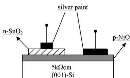
Fig. 1. Schematic drawing of the n-SnO<sub>2</sub>/p-NiO heterojunction grown on (001) p-Si substrate.
