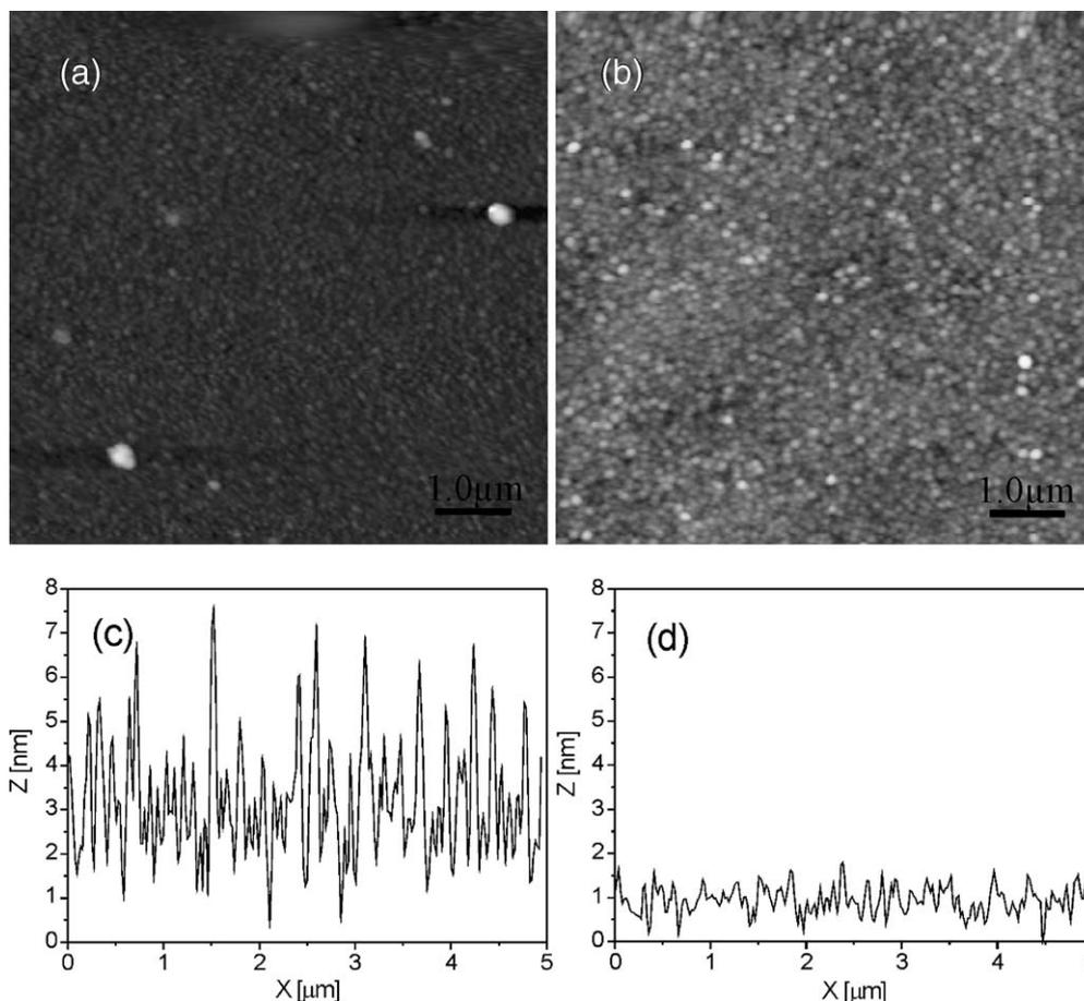
Fig. 2. AFM images and surface profiles of ZnO films with Au coverage obtained with (a and c) 300 and (b and d) 9000 laser pulses used for the irradiation of the Au target.
