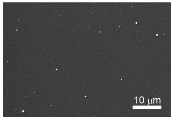
Fig. 1. SEM image of ZnO film with Au coverage obtained with 9000 laser pulses used for the irradiation of the Au target.
