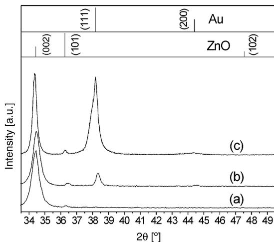
Fig. 3. X-ray diffractograms of ZnO films with Au coverage deposited with (a) 300, (b) 600, and (c) 9000 laser pulses used for the irradiation of the Au target, as well as diffraction patterns of hexagonal ZnO and cubic Au as referred in the JCPDS 36-1451 and 04-0784 files, respectively.
