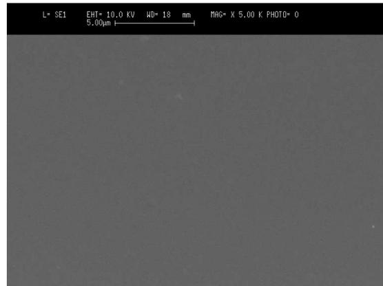
Fig. 3. SEM image of a thin film deposited in vacuum by the two synchronised lasers system. The UV and IR laser fluences were  $0.75$  J/cm<sup>2</sup> and  $8$  J/cm<sup>2</sup>, respectively. The time delay between the UV and IR laser pulses was 200  $\mu$ s. The mark corresponds to 5  $\mu$ m. The complete elimination of particulates is evident.
