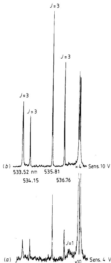
**Figure 3.**  $J$  level identification of the resonance lines in the  $Sr^+$  spectrum allowed by the comparison of spectra recorded with: (a) linearly polarised laser beam (laser pulse energy: 1.8 mJ); (b) circularly polarised laser beam (laser pulse energy: 2 mJ). Note that for this particular recording the laser beam has been focused with a lens of 200 mm focal length in order to minimise depolarisation effects and make easier the recognition of selection rules.
