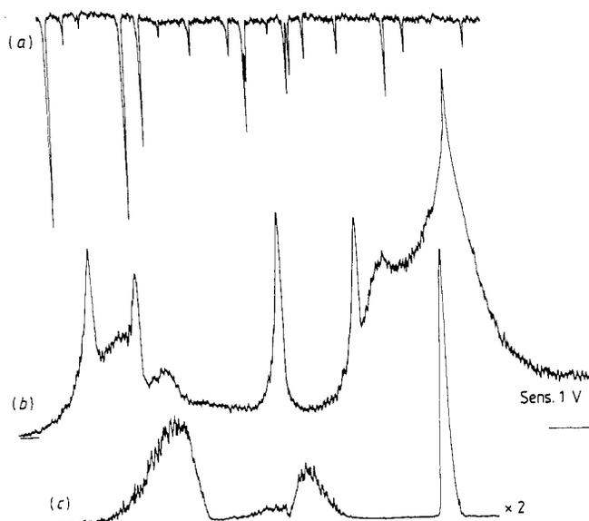
**Figure 5.**  $\text{Sr}^+$  and  $\text{Sr}^{++}$  yield spectra recorded for an energy of 0.9 mJ per light pulse with linearly polarised light: (a) Ne hollow-cathode OG spectrum for wavelength calibration; (b)  $\text{Sr}^+$  yield; (c)  $\text{Sr}^{++}$  yield.
