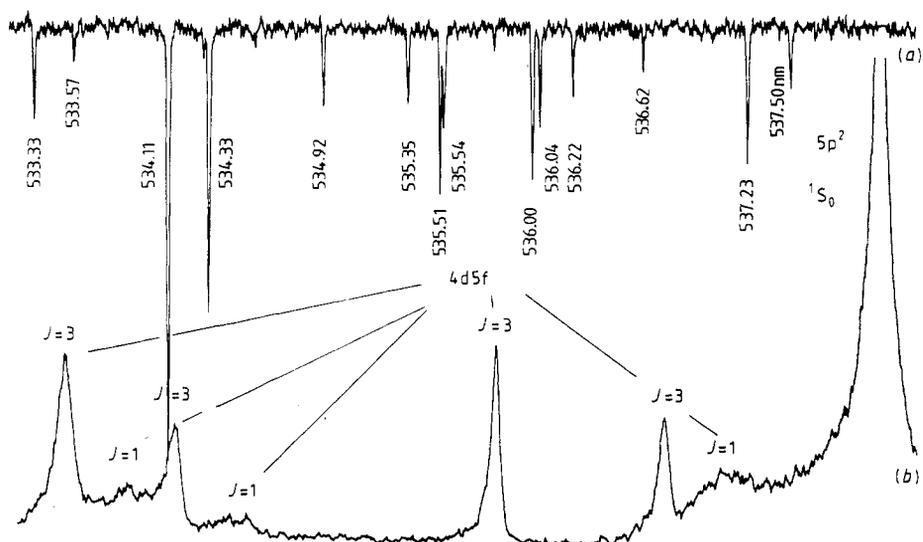
**Figure 2.** Sr<sup>+</sup> yield spectrum between 533 and 538 nm with linearly polarised light: (a) Ne hollow-cathode OG spectrum for wavelength calibration; (b) Sr<sup>+</sup> signal as a function of laser wavelength.
