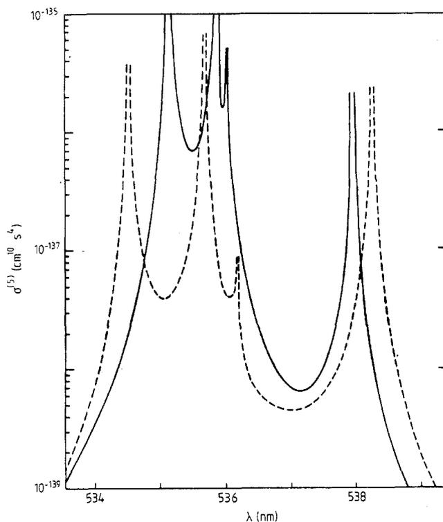
**Figure 6.** Intensity-dependent five-photon ionisation cross sections from the  $5s_{1/2}$  state of  $\text{Sr}^+$  for two intensities: full line, intensity lower than  $1 \text{ GW cm}^{-2}$ ; broken line, intensity  $15 \text{ GW cm}^{-2}$ . For increasing wavelength, resonances occur in the order  $6p_{3/2}$ ,  $7d_{5/2}$ ,  $7d_{3/2}$ ,  $6p_{1/2}$ .
