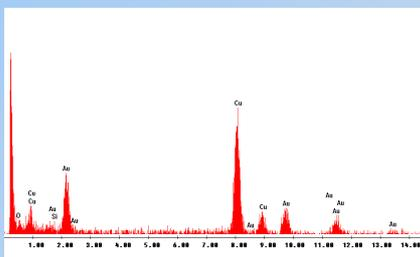
The EDX spectrum provided evidence for the presence of Au nanoparticles on the surface of the Cu<sub>x</sub>O/SiO<sub>2</sub> thin film.
