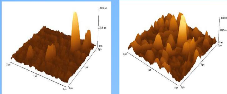
The substrate type had an effect on the surface morphology of the films; the one on SiO<sub>2</sub> substrate was smoother than the other on glass substrate.
