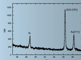
**Figure 4.** XRD spectrum of a ZnO thin film on which Au was subsequently deposited for 5 min. Besides the Si (substrate) and ZnO peaks, the Au peak at 38.5 $^{\circ}$  appears indicating the growth of Au clusters on the film surface.
