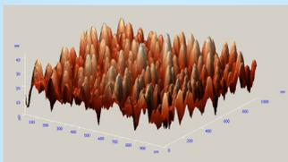
**Figure 2.** The AFM picture shows an as-deposited thin ZnO film grown on oxidized silicon wafer. The average grain size of around 30-40 nm is not affected by the annealing process due to the low (400 $^{\circ}$  C) temperature used. The indicated high surface-to-volume ratio favors the application of such films as gas sensors since the chemical active area is enhanced.
