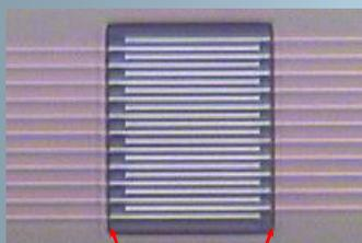
**Figure 1.** Scanning Emission Microscopy image showing the ZnO field-effect gas sensor. Intra-electrode distance is 1  $\mu\text{m}$ . The ZnO film is seen in the middle.
