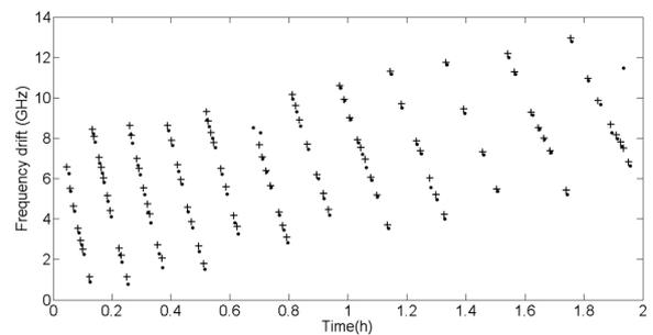
Fig. 3: Plot of the rate of the frequency drift vs the elapsed time from the moment the laser started to operate.
