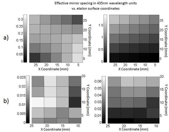
Fig. 7: Right: Map of the effective etalon spacing in units of 435 nm wavelength (gray scale) . Left: Map of the effective etalon spacing with deviation from parallelism removed to reveal the etalons flatness. a) Prototype 13 mm etalon b) Commercial 5 mm etalon.
