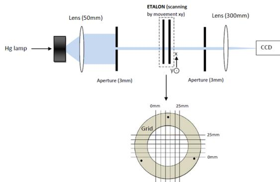
Fig. 6: Experimental setup for the characterization of the Fabry-Perot etalon with respect to its Flatness.
