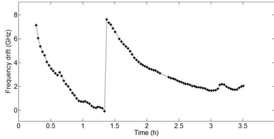
Fig. 4: Plot of the relative Frequency of the most intensive laser mode vs. the elapsed time from the moment the laser started to operate.
