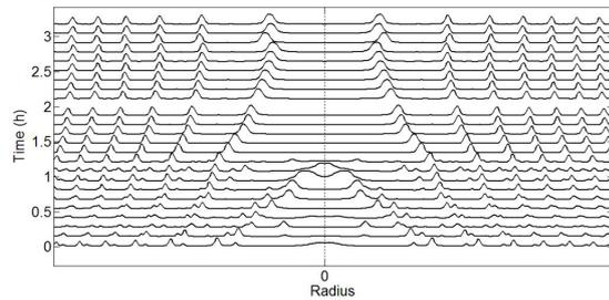
Fig. 5: One dimensional intensity plots of the fringe patterns shifted at an amount equal to the time they were taken.
