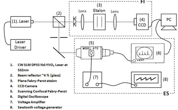
Fig. 2: The experimental setup for the characrerisation of the Nd:YVO<sub>4</sub> Laser.
